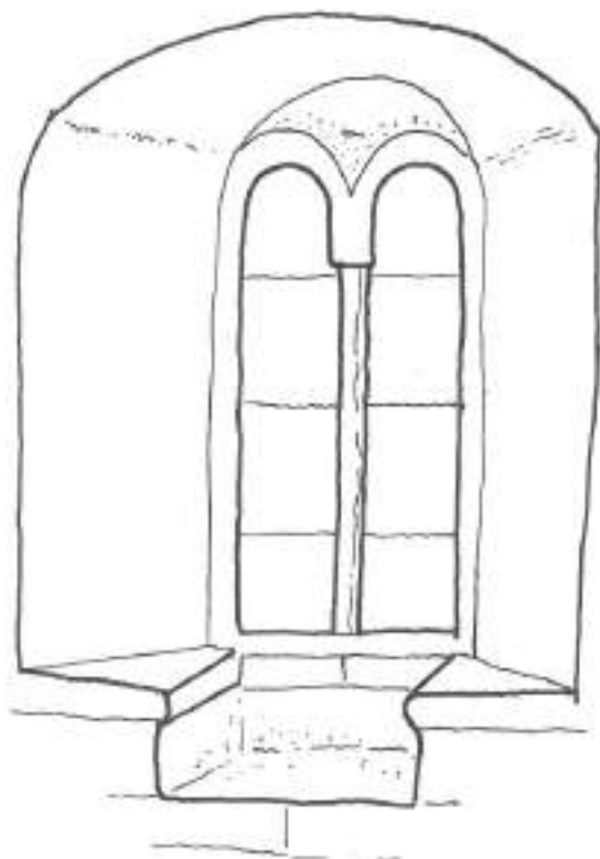
Norman two-light window with deep splay and window seats.
